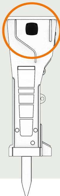
Locate safe mounting spot on your tool that both ensures good signal conditions and lessens the risk of impact from debris.
