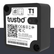
**T1** is a small IoT tracking device and data logger designed for **data tracking and monitoring** of any asset – stationary or moving – where certain data or conditions are essential for compliance or safety.
