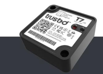
**T7** is a small IoT tracking device and data logger that offers **asset monitoring and data tracking** of any asset; from non-powered equipment to entire fleets.
