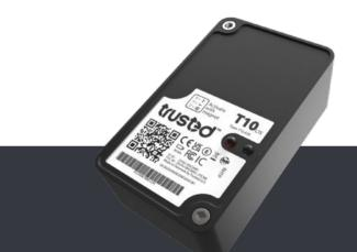
This **RHTP** edition features high precision **humidity**, **temperature and air pressure** monitoring in one device.
