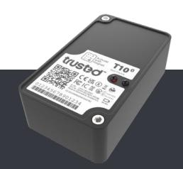
**T10 Bluetooth®** is an IoT tracking device and data logger designed for **data monitoring and tracking** of assets like hydraulic attachments and sensitive freight.
