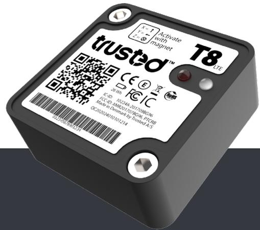
T8<sub>LTE</sub> is a unique IoT product featuring the low power communication technology LTE Cat-M1. It typically offers 5 years battery lifetime based on 1 position/day.
