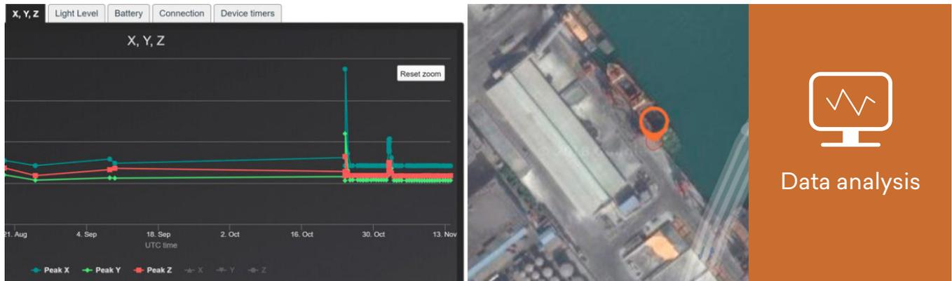
Logged data on shock levels, as displayed in the graph seen above, indicates that the cargo had been handled with caution until it reached the port. Here the container received an impact of 5,5 G – indicating a drop.
